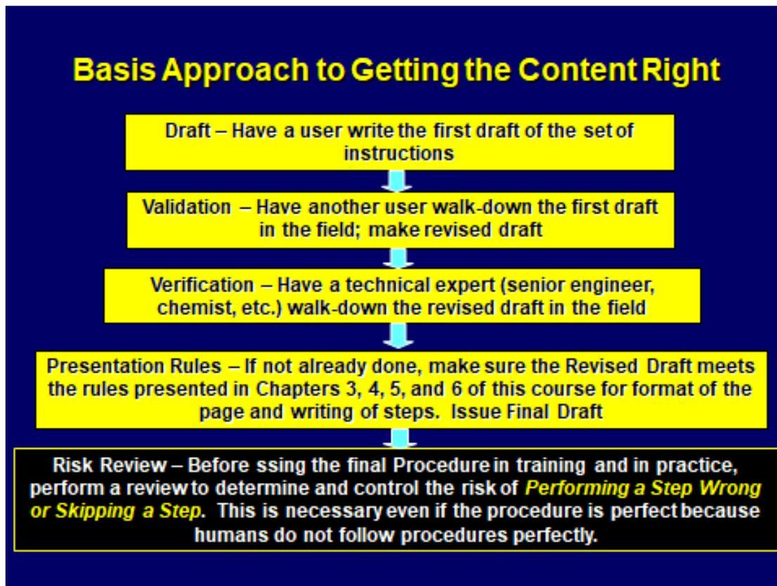
Figure 1. Best Approach to developing written procedures, once the unit has decided which procedures are needed (Extracted from PII Course, Writing Effective Operating and Maintenance Procedures © PII 2003-2017)<sup>[6]</sup>
