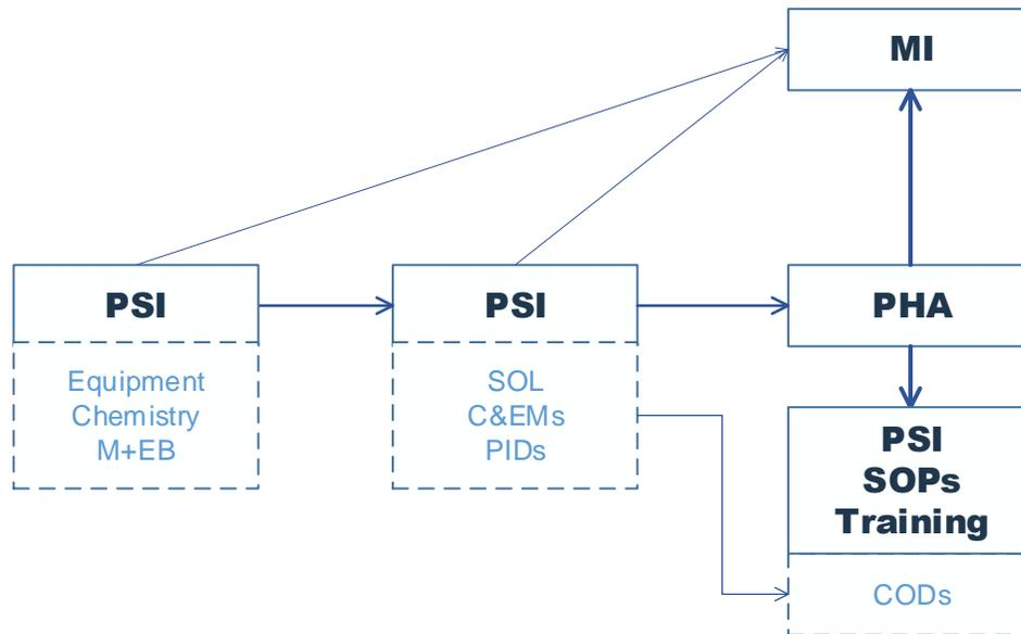
**Figure 3. Relationship of Specific PSI to PHAs, MI, SOP and Training**
