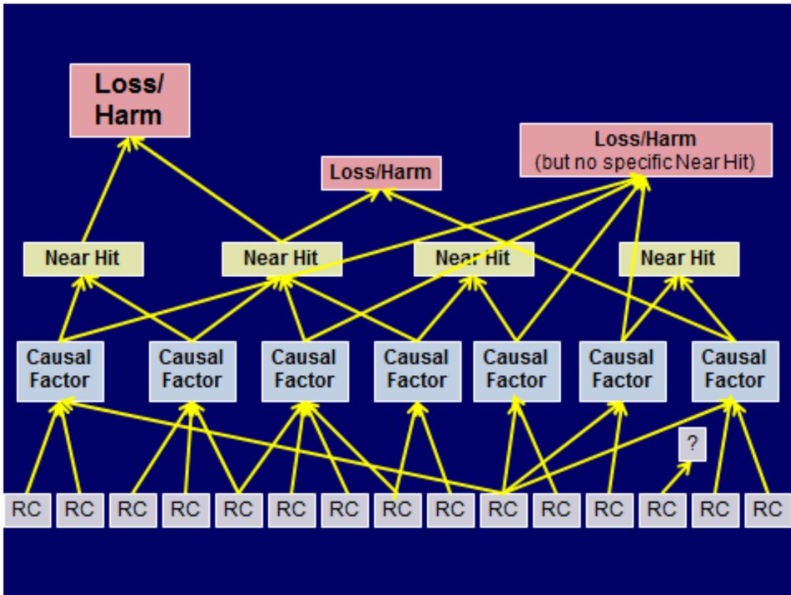
**Figure 1 Interrelationship between the causes of Accidents (Losses) and the causes of Near Misses**
