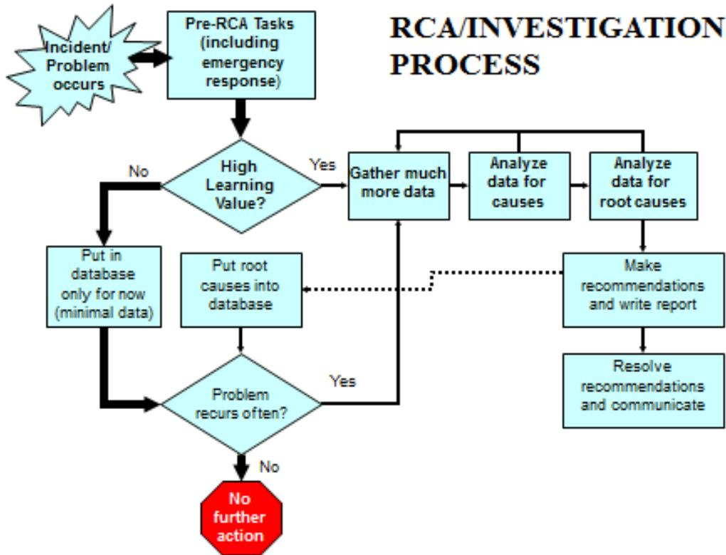
**Figure 2: RCA/Investigation Flow Process**
